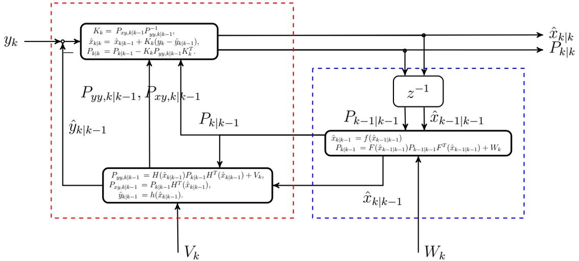
Figure 2: EKF block diagram. Time-update and measurement-update blocks are represented by blue and red dashed rectangular.
