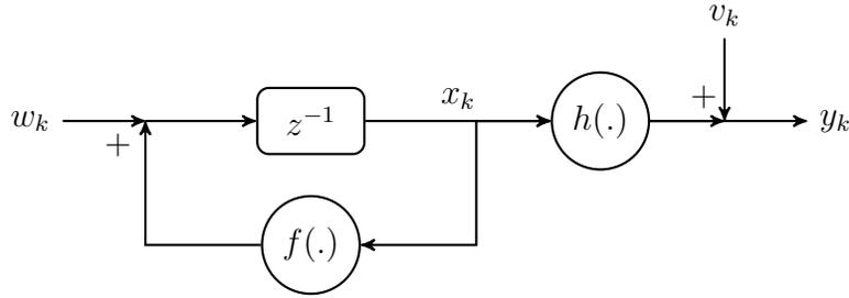
Figure 1: Block diagram of the nonlinear state space model (1).
