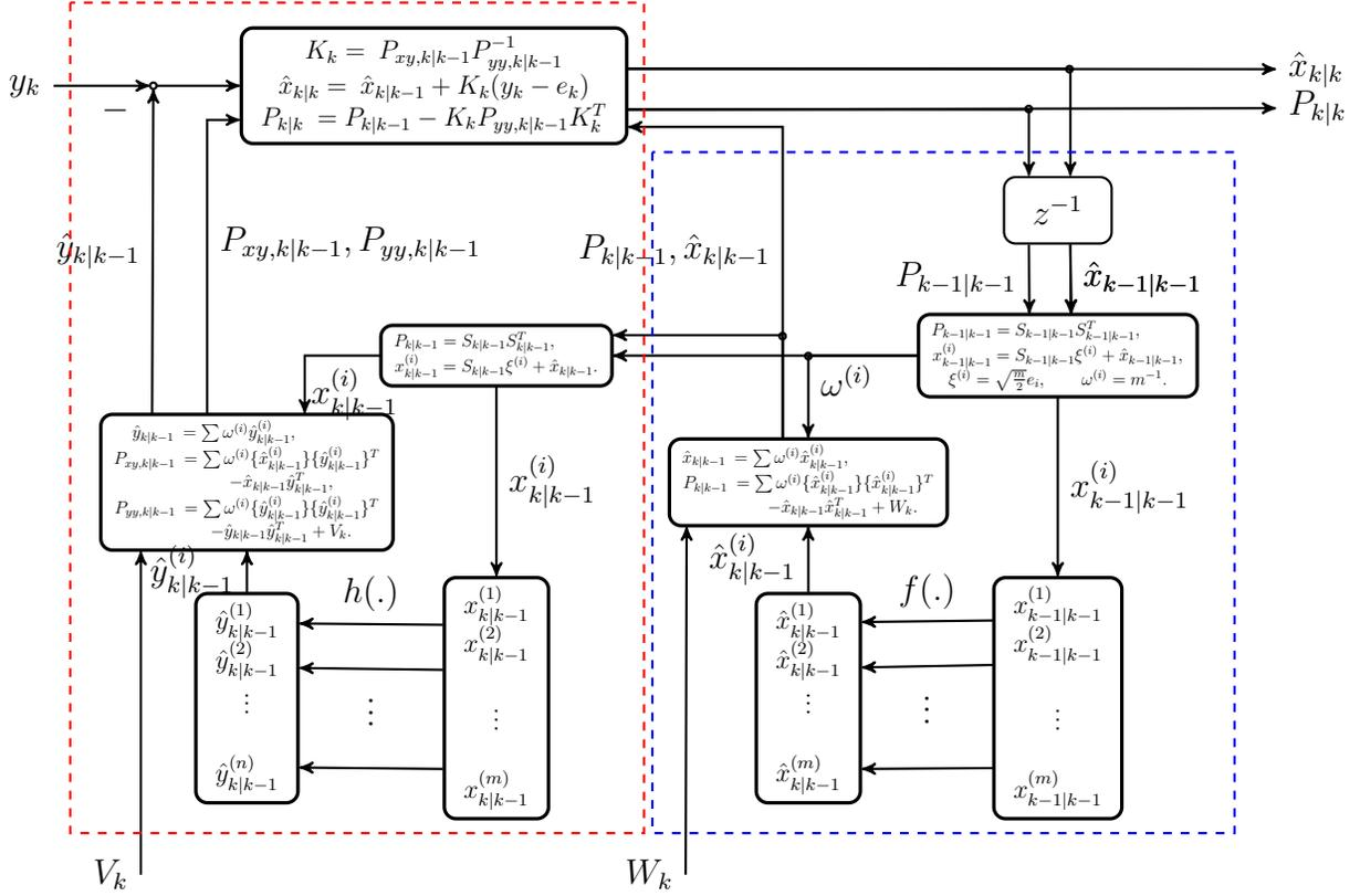
Figure 3: CKF block diagram. Time-update and measurement-update blocks are represented by blue and red dashed rectangular.
