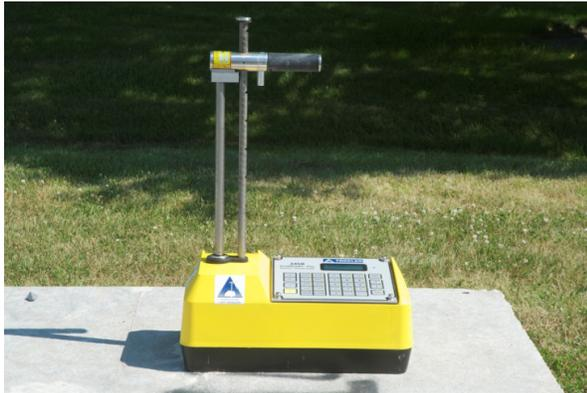
**Fig. 2.** Nuclear Density Gauge on Field Specimen 2-1.**Table 7. Neutron Measurements of Field #2**
