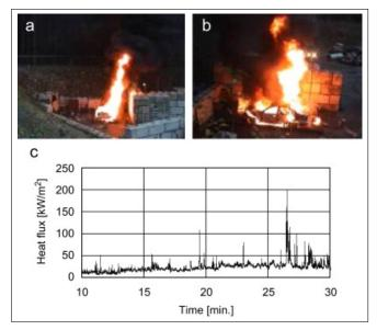
Fig. 13. Gasoline flame from a vehicle filled with 40-L tank. (a) back view, (b) side view, (c) graph of heat flux with respect to time [15].
