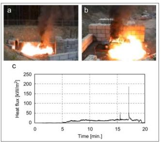
Fig. 15. Downward hydrogen flame from vehicle with two 35MPa installed. (a) back view, (b) side view, (c) heat flux with respect to time [15].
