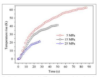
Fig. 20. Temperature rise with different initial pressure in the cylinder [9].
