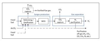
Fig. 2. The route for hydrogen production from fossil fuel sources with  $CO_2$  capture. Solid black lines represent gasification or reformation processing. The dash black lines represents other streams or processing such as methane reformation processing [16].
