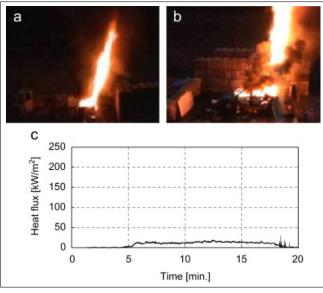
Fig. 14. Upward hydrogen flame from a vehicle with two 35MPa installed. (a) back view, (b) side view, (c) heat flux with respect to time [15].
