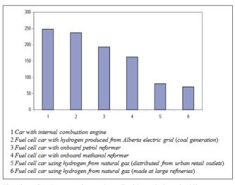
Fig. 6. Graph comparing carbon dioxide emissions in kilograms per 1000km of cars, using different types of fuel sources [22].
